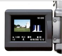
The LCD screen on the Canon PowerShot G2 shows a screen with camera settings, a histogram, and a thumbnail image.
