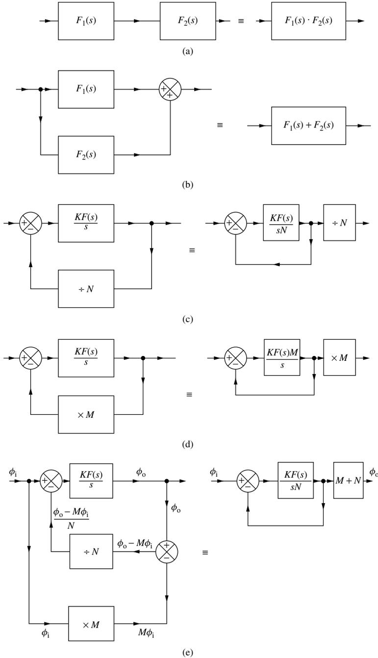
**Figure 1.5** Simplification of the block diagrams of PLLs: (a) series connection; (b) parallel connection; (c) and (d) feedback arrangement; (e) more complicated system. (Reproduced from Fig. 1.20 in C.J. Savant Jr., *Basic Feedback Control System Design*. New York, Toronto, London: McGraw-Hill, 1958 by permission of McGraw Hill, 2002).
