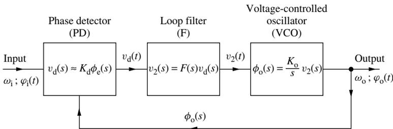
**Figure 1.3** Simplified block diagram of the PLL with individual transfer functions.
