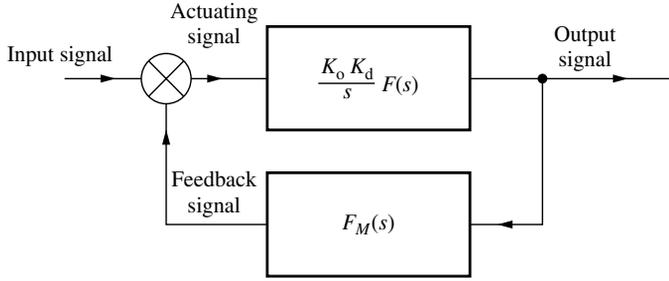
**Figure 1.4** Simplified block diagram of the PLL with a transfer function in the feedback path.
