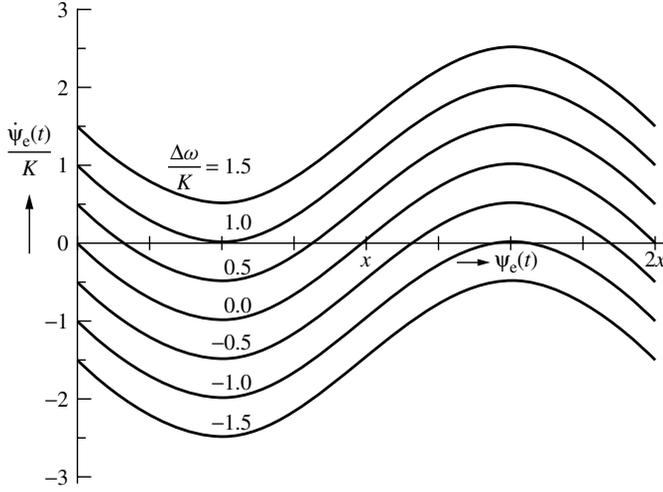
**Figure 1.2** Plot of relation (1.10) in the phase plane for different ratios  $\Delta\omega/K$ .
