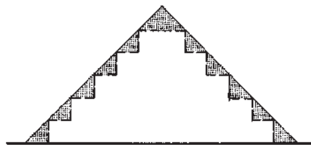
Figure 1.4. Surface smoothing between adjacent contour lines.
