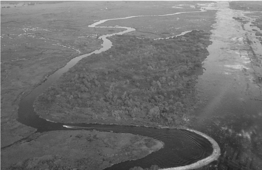
Figure 1.2 Part of the Everglades area restoration has involved the remeandering and restoration of the Kissimmee River that flows from central Florida to Lake Okeechobee. At approximately 10 times the cost of the stream straightening that occurred in the 1960s, the river is being partially restored by low-head dams and reattachment of backwaters and old meanders to the stream channel. (Courtesy of Lou Toth; photo by Paul Whalen, South Florida Water Management District, West Palm Beach, Florida; reprinted with permission.)
