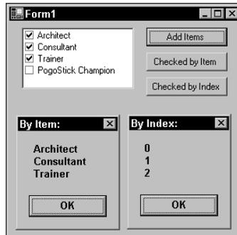
**Figure 2.8** Items in a CheckedListBox can be interrogated for their checked status by Index or by Item.
