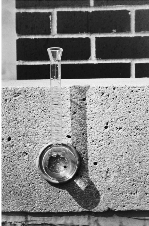
FIGURE 2.17 A simple test using a plastic tube adhered to the surface with soft putty provides quantitative information on how fast a material will absorb water. For more information about this water absorption test, see: Kim Basham and John Meredith, "Measuring Water Penetration," Masonry Construction Magazine (November 1995): 539. Photo by G. Russell Heliker.
