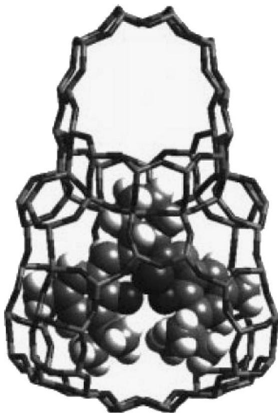
Figure 1.13 The ‘ship-in-a-bottle’ concept: view of Mn(III)–salen inside the cavity of zeolite EMT. Reproduced from Ogunwumi and Bain [138] by permission of Royal Society of Chemistry
