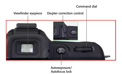
**1.11** Key components on the upper-right corner of the back panel of the D50.
