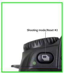
**1.10** Key component on the upper-left corner of the back panel of the D50.
