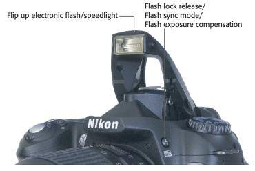
**1.4** Pressing the flash multi-button (Flash Exposure Compensation button) pops up the built-in electronic flash, ready for use.
