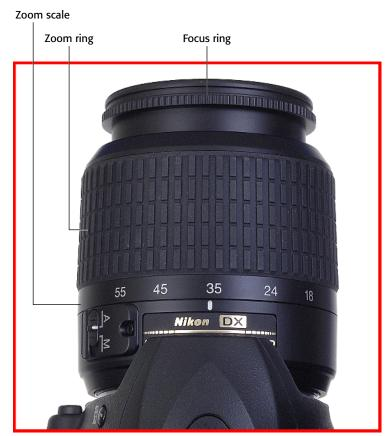
1.6 Key components of a typical zoom lens.
