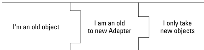
Figure 1-5: Old objects work with new objects via an adapter.
