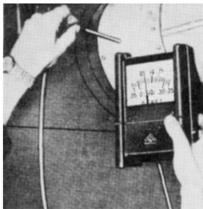
Figure I-45 Bacharach model MZF draft gauge.
