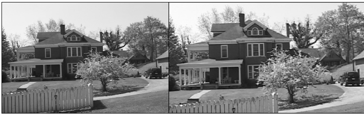
Figure 1-12: 16:9 video on a DV camcorder (on the right) isn't really widescreen as much as stubby screen. As you can see by comparing it to the full resolution DV on the left, the camcorder simply cuts strips from the top and bottom of the video.
