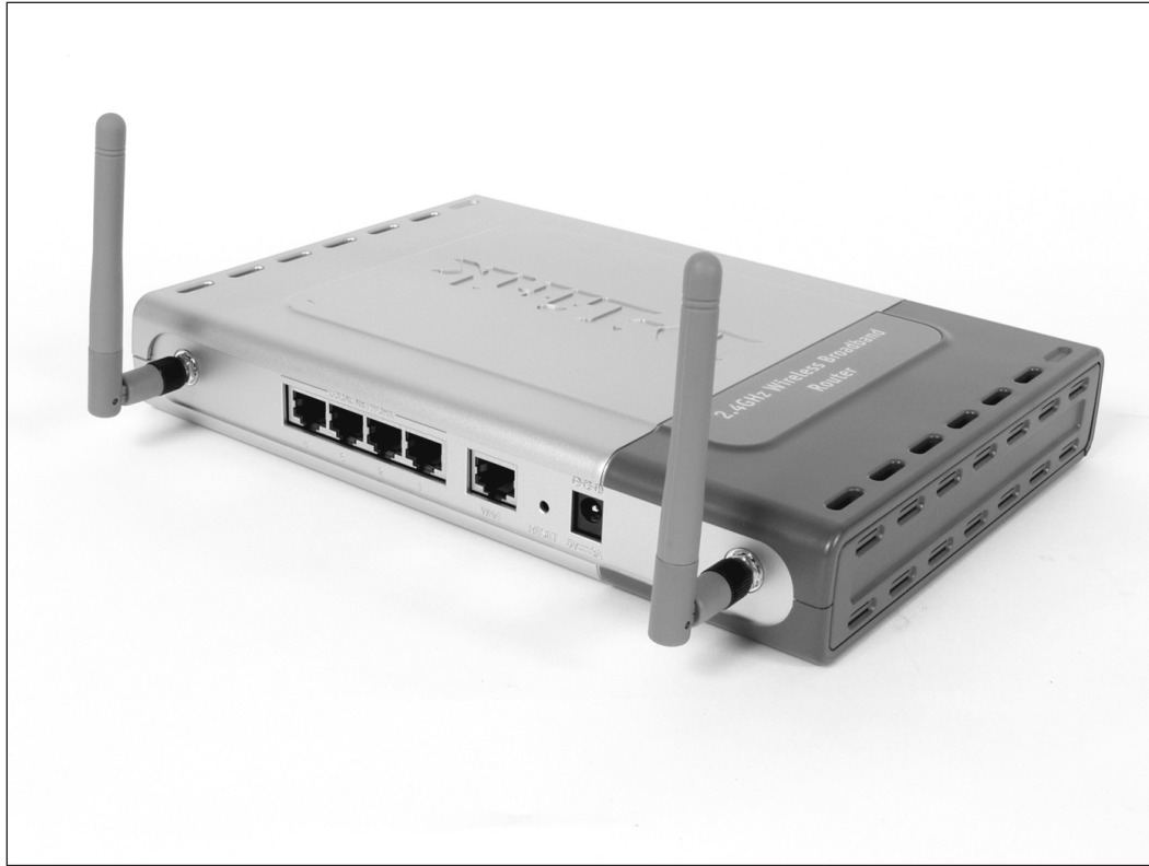
Figure 1-3: D-Link calls its model DI-624 a Wireless Broadband Router. It combines a four-port Ethernet switch, a wireless access point, and a firewall into one compact, inexpensive unit.
