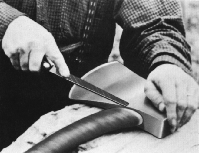
Figure I-22 Using one hand to do light filing. (Courtesy Nicholson File Company.)
