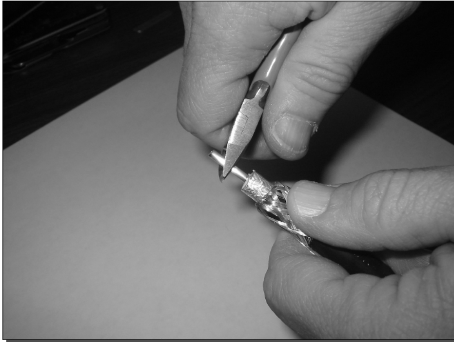
FIGURE 1-18: Clipping the core conductor.
