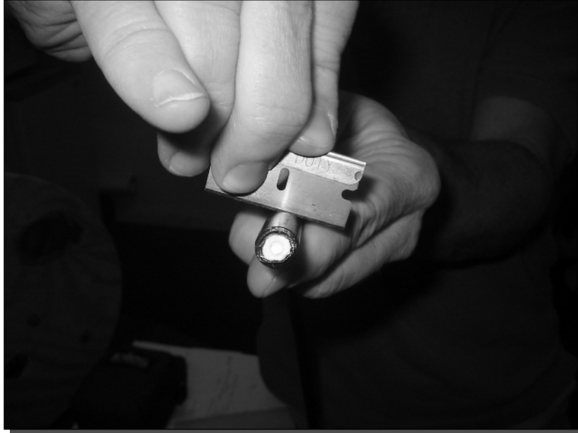
FIGURE 1-12: Stripping using a rocking motion. Watch those fingers!
