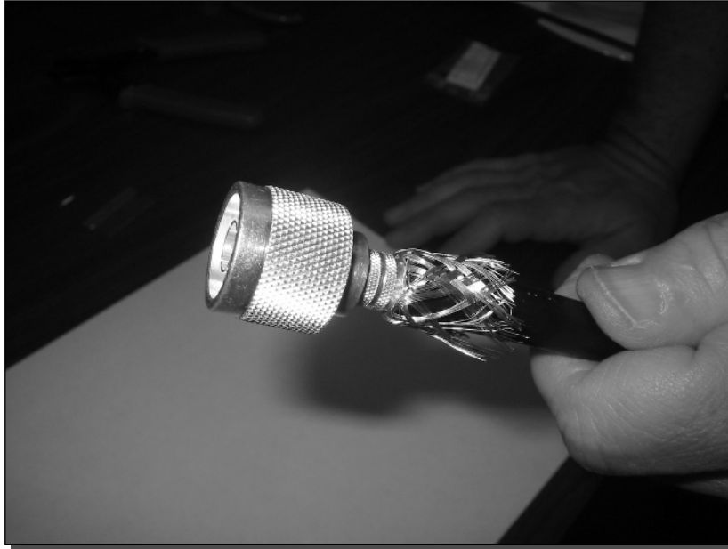
FIGURE 1-22: Connector and pin are in position.
