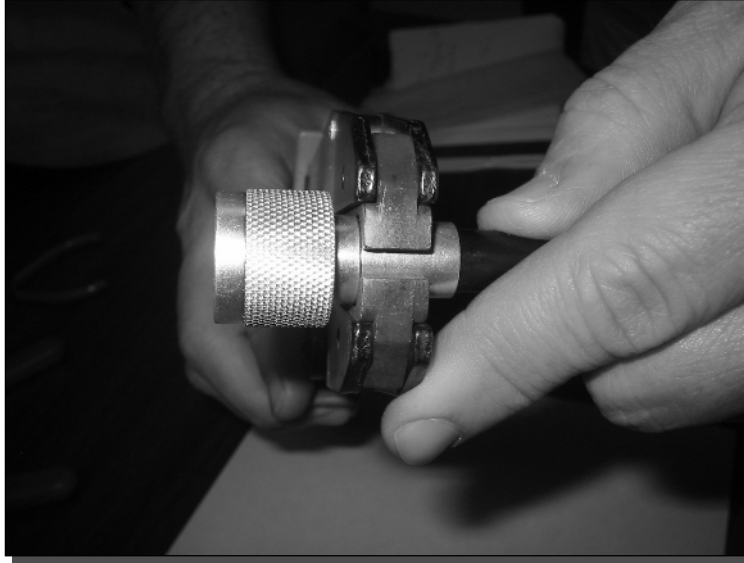
FIGURE 1-25: Crimping the crimp ring onto the cable.
