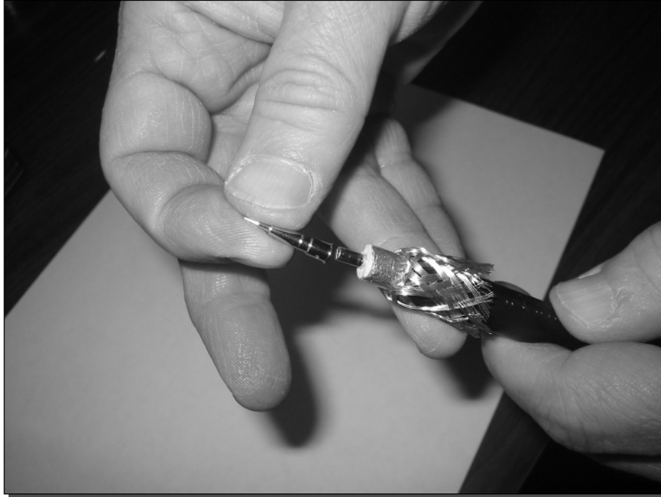
FIGURE 1-19: Placing the center pin onto the conductor.
