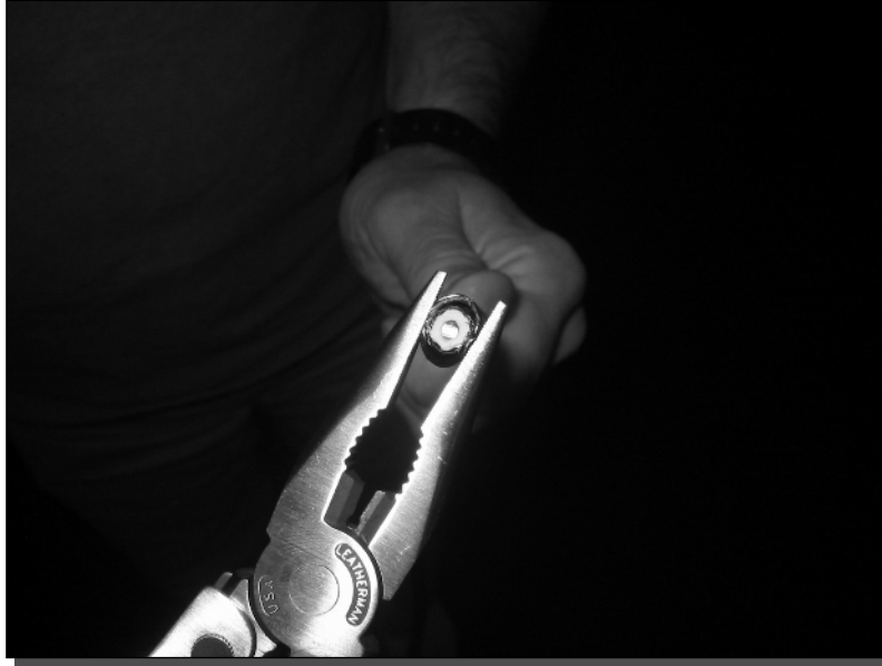
FIGURE 1-10: Using pliers to reform the white foam core.
