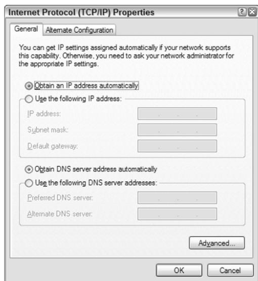
**Figure 3-9:** Configuring the TCP/IP settings.
