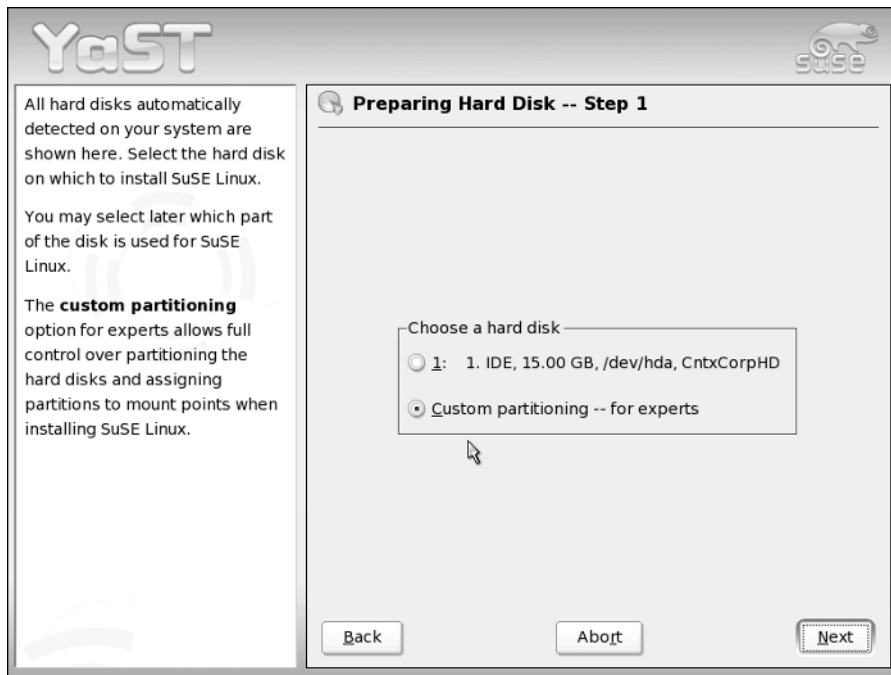
Figure 1-8: Selecting custom partitioning
