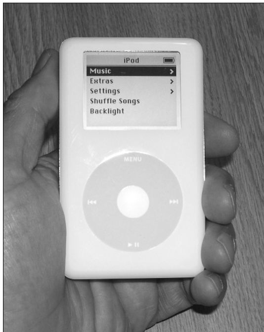
Figure 1-3: The fourth-generation iPod uses the same click wheel as iPod mini.
