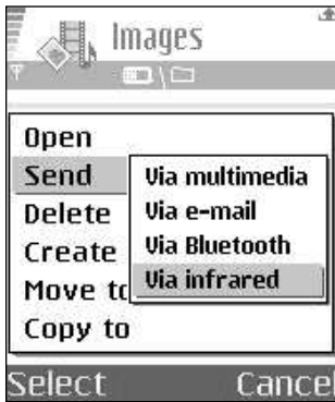
Figure 1-18: Choose Via Infrared to send the image directly to another phone via a wireless connection.
