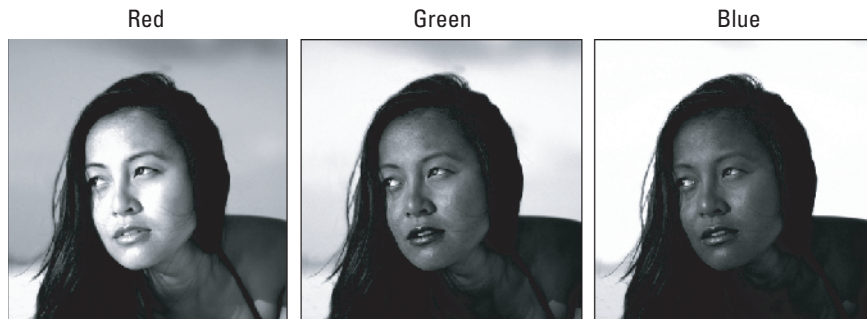
Figure 4-17: Of the three color channels, the blue channel offers the best contrast between hair and background.
