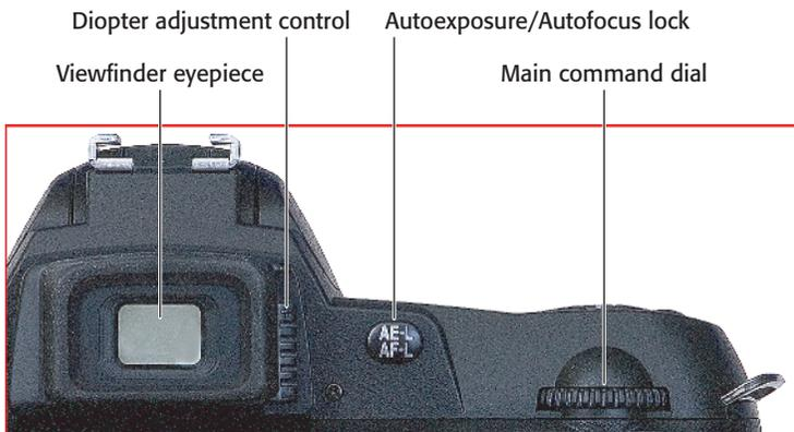
**1.11** Key components on the upper-right corner of the back panel of the D70.
