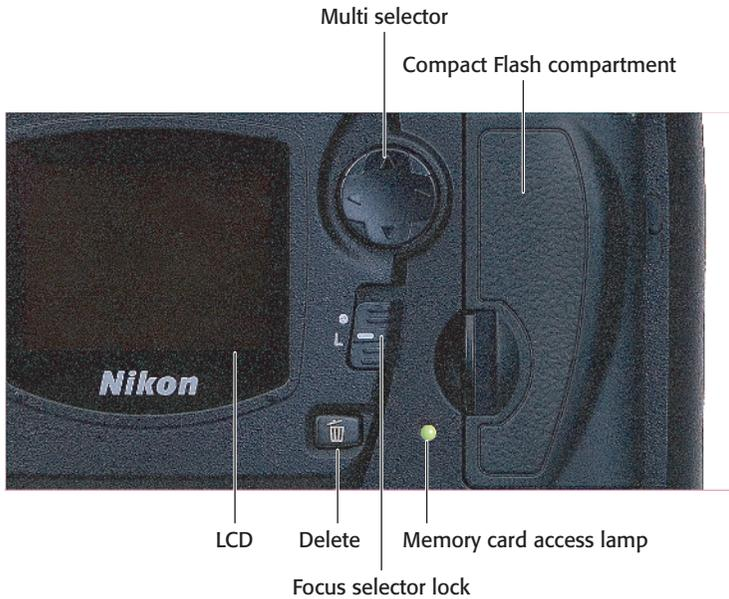
**1.13** Key components on the lower-right corner of the back panel of the D70.
