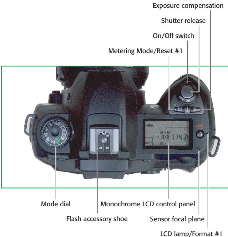
1.8 Key components on the top panel of the D70.
