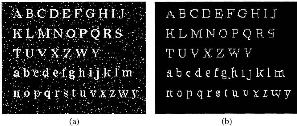
Figure 1-17. Realization of Fig. 1-16(a) with 5% random pepper noise and the result of the designed iterative filter after four iterations.
