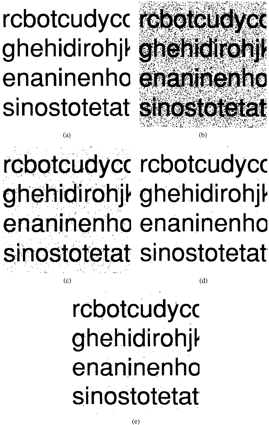
Figure 1-15. Text restoration: (a) ideal realization; (b) degraded realization; (c) restoration with single-stage W -filter; (d) restoration with two-stage W -filter; (e) restoration with single stage (W \oplus W) -filter.
