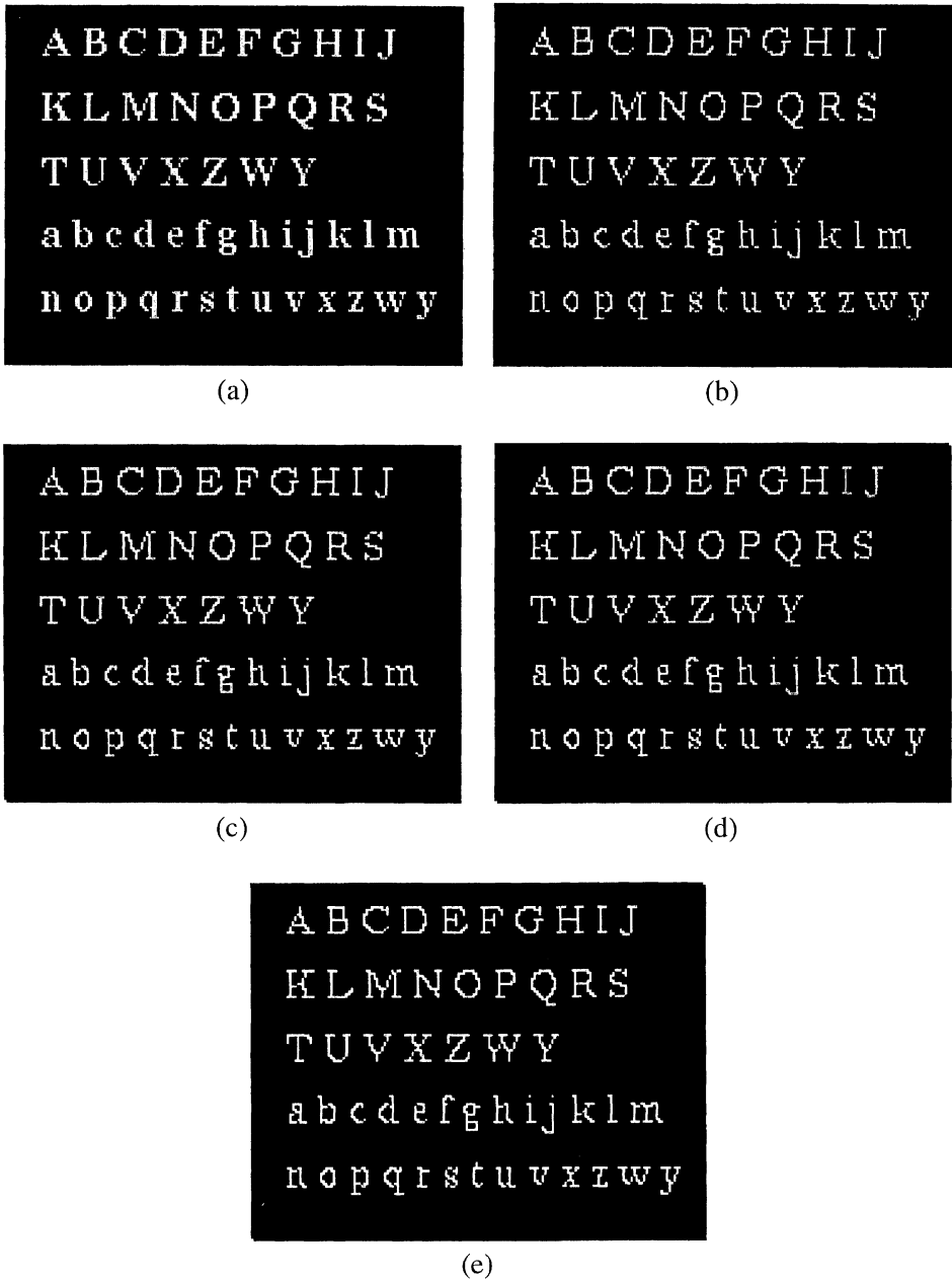
Figure 1-16. Connected thinning: (a) realization of input process; (b) result of first iteration; (c) result of second iteration; (d) result of third iteration; (e) result of fourth iteration.
