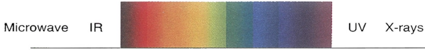
Figure 1.2 The visible spectrum is in the range from 0.7 \mu\text{m} (700 nm) to 0.4 \mu\text{m} (400 nm). The yellow light of a sodium lamp has a wavelength of 589 nm.
