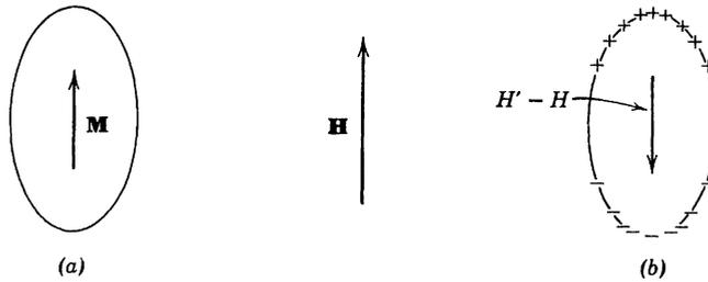
Fig. 1-5.1. (a) A uniformly magnetized ellipsoid and (b) the equivalent poles. The uncompensated surface poles produce a uniform internal field  $H' - H$  and an external field that is identical to that of an equivalent dipole positioned at the ellipsoid's center. **H** is a uniform applied field.
