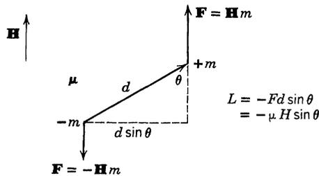
Fig. 1-10.1. Torque on a dipole produced by an external field  $H$ .
