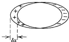
Fig. 1-5.2. Uncompensated charges or poles for two ellipsoids of opposite charge densities and a distance  $\delta x$  apart.
