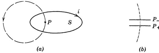
Fig. 1-7.2.  $S$  is the shell with wire-carrying current  $i$  as its boundary. For simplicity the shell is considered to be plane. The dotted curve is the path along which a unit pole is taken. (b) shows the points  $P_+$ ,  $P_-$  at which the path crosses the shell of definite although infinitesimal thickness.
