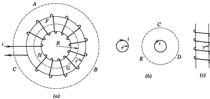
Fig. 1-7.1. The toroid is shown from above in (a) and in a vertical cross section in (b). The result when  $R \rightarrow \infty$  is the solenoid shown in (c).
