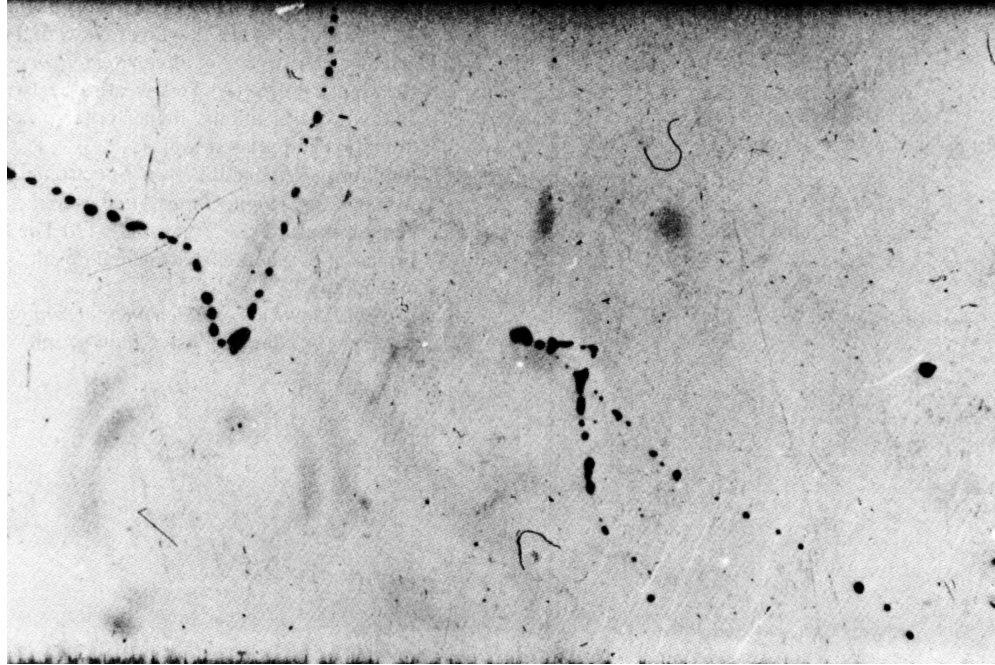
Fig. 1: Photoelectrons and Auger electrons from krypton ionized with 60-keV x rays, photographed in a cloud chamber by Pierre Auger ca. 1923. (Courtesy P. Auger).
