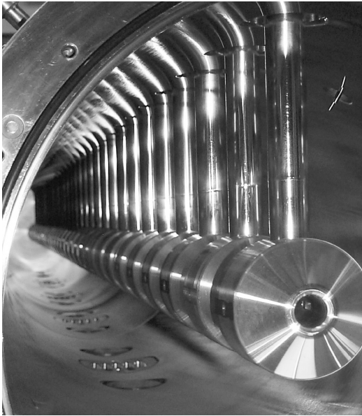
Fig. 2: Cut-away drawing of a 402.5-MHz 4.2-m 60-cell drift-tube-linac structure at the Spallation Neutron Source (SNS) at Oak Ridge National Laboratory. The photograph shows copper drift tubes and the drift-tube support stems.
