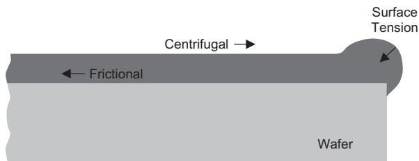
Figure 1.15 A balance of spin-coat forces at the wafer edge leads to the formation of a resist edge bead
