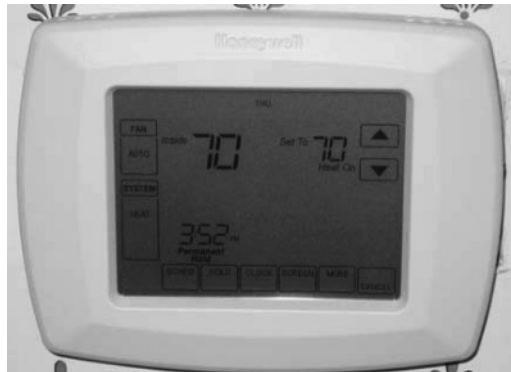
Figure 1.5 This thermostat offers larger controls and display, making it easier for older individuals.
