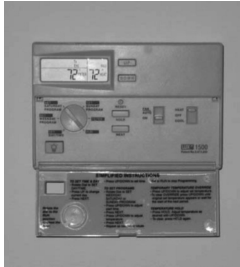
Figure 1.4 A thermostat that offers the needed functionality, but is too small to read and accurately control.
