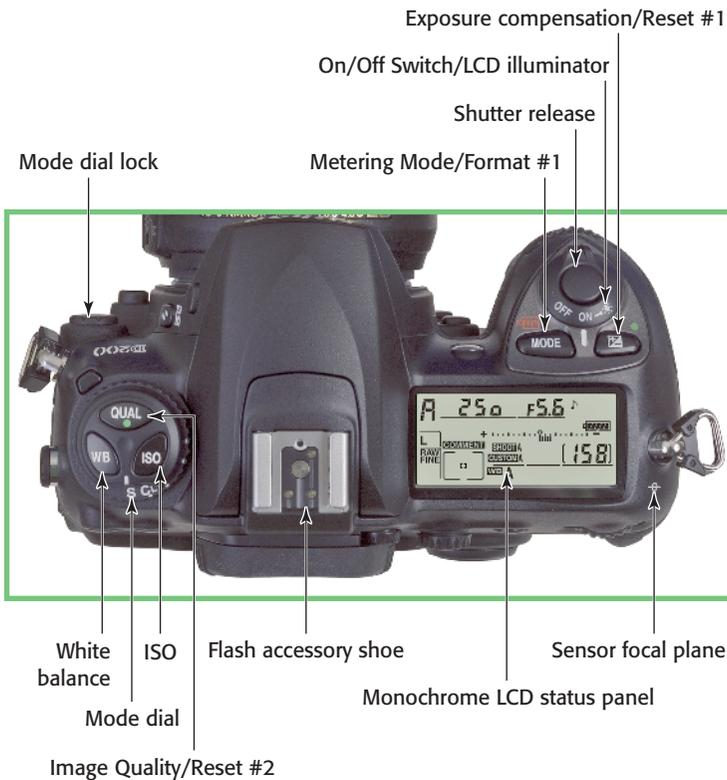
1.8. Key components on the top panel of the D200.
