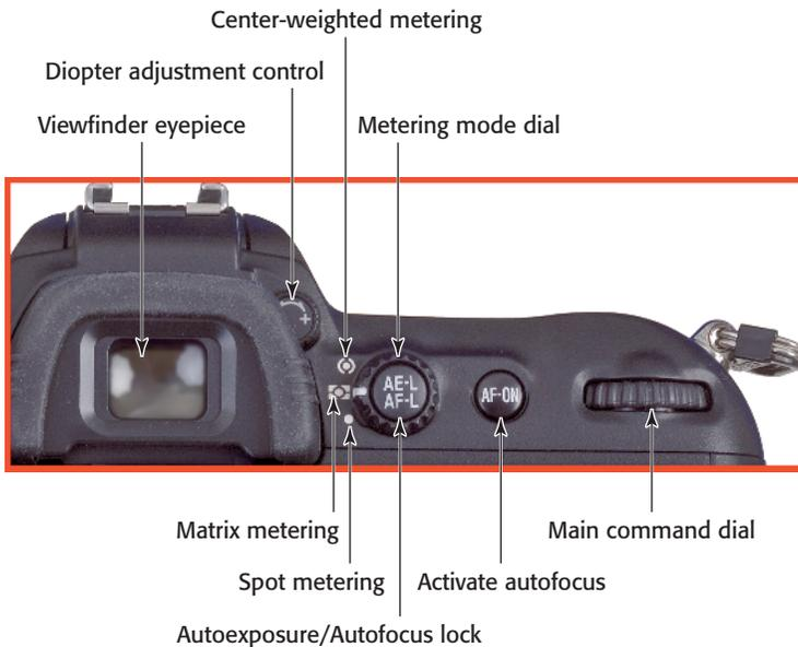
**1.11** Key components on the upper-right corner of the back panel of the D200.
