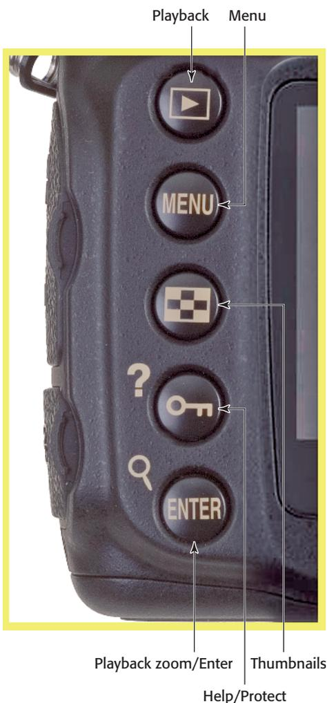
**1.12** Key components on the lower-left corner of the back panel of the D200.
