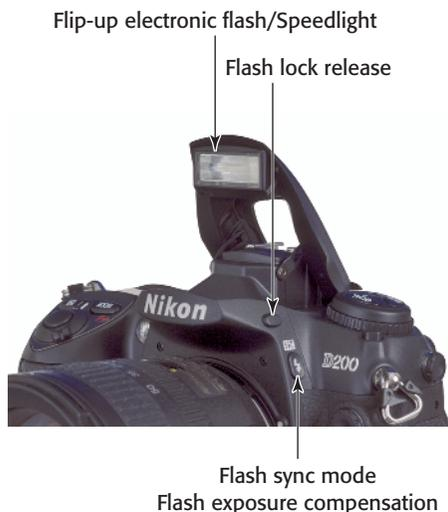
**1.4** Pressing the flash multi-function button (flash exposure compensation button) pops up the built-in electronic flash, ready for use.
