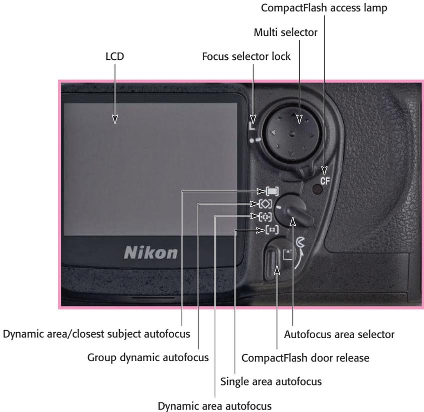
**1.13** Key components on the lower-right corner of the back panel of the D200.
