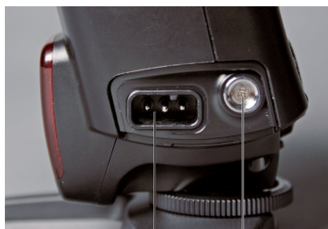
1.4 External power supply terminal (left) and Speedlite bracket fitting (right)
