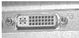
FIGURE 1.13 One of several possible DVI connectors
