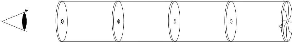
Figure 1.4 A long tube with internal baffles and an adjustable aperture. When observers view colored patches through such a tube, the patches look grayish-white. When the entire Mondrian is viewed, the patches appear to have a color that corresponds to the reflectance properties of the patch.
