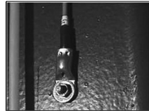
Temp. sensor fastening detail
