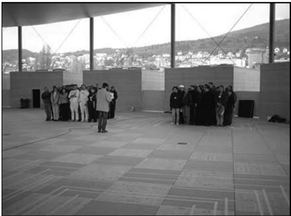
People standing on representative locations simulating concentrated load
