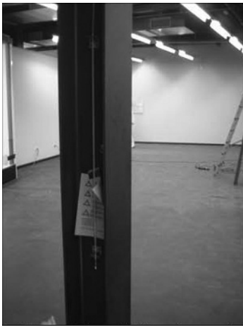
Sensor fastened to the column web
