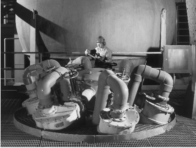
FIGURE 1-13 A set of hydrocyclones, which is used for effective desliming, i.e., removal of insoluble particles, from potash ore.
