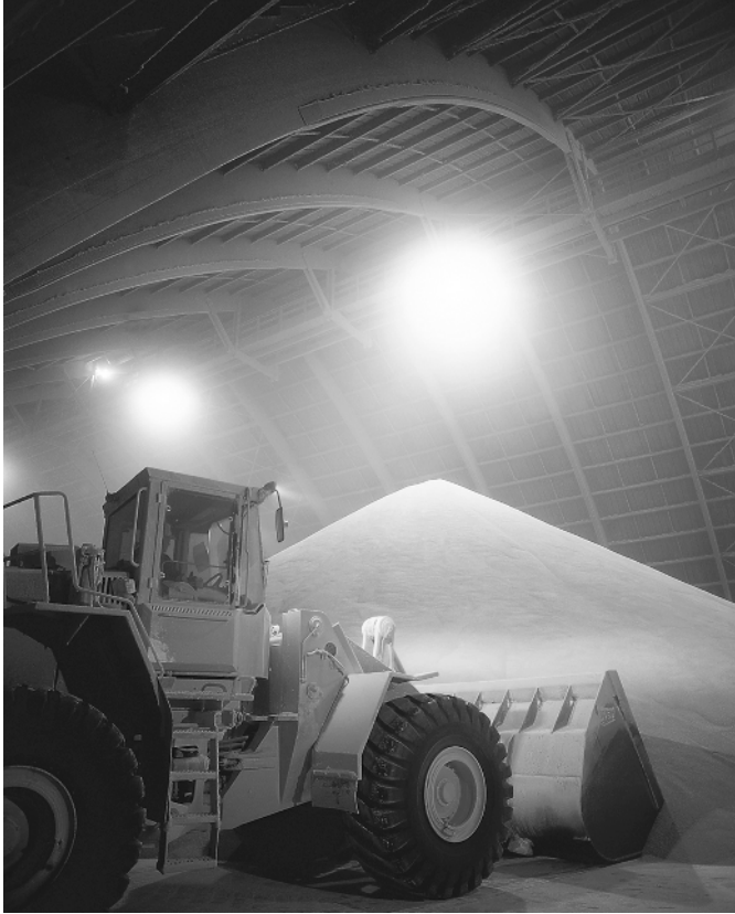
FIGURE 1-20 A storage facility containing potash product. In the foreground is a loader, which is used for moving the product to a reclaim conveyor, which transports the product to the loading facility.
