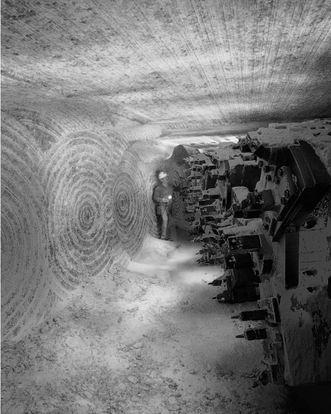
FIGURE 1-1 A potash miner inspects the front of a continuous boring machine. Machines such as this unit will cut up to 700 metric tons of ore per hour from the ore body and deposit it on a conveyor belt for transport to the shaft.
