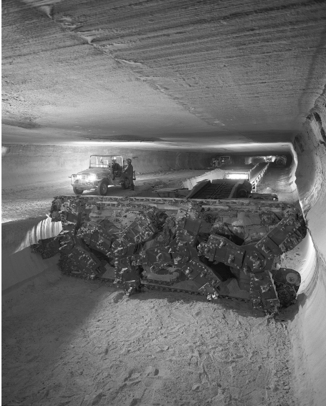
FIGURE 1-7 Photo of a 4-rotor continuous mining machine at PCS Potash, Lanigan. The long room-and-pillar mining method is utilized at Lanigan; completed 4-pass mine rooms are 42' wide and 16' high. An extensible conveyor belt is located behind the mining machine; the ore is transported back to the shaft by conveyor belt and then hoisted to the surface.
