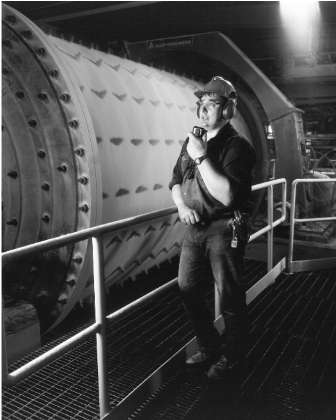
FIGURE 1-12 A potash plant operator standing beside a rod mill, used for the secondary comminution of potash ores.
