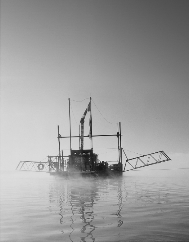
FIGURE 1-10 Harvesting KCl from the bottom of a cooling pond using a dredge, at the PCS Patience Lake mine.
