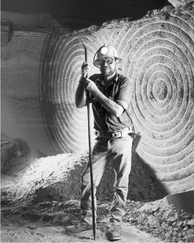
FIGURE 1-3 A potash miner stands in front of the sylvinitic ore face, which shows the characteristic circular grooves cut into the ore by the tungsten carbide bits on the mining machine rotors. The miner is holding a scaling bar, which is used to inspect the roof for loose rocks and safely remove them. Mounds of potash ore, recently extracted from the face, lie on the floor behind the miner.
