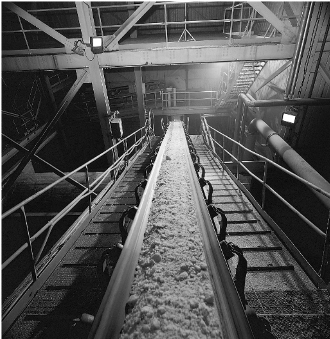
FIGURE 1-11 Transportation of potash ore from the skips (hoist) to the ore storage bin. Processing potash ore involves moving hundreds (or thousands) of tons of material from one part of the process to the next; conveyor belts are one of the common pieces of equipment used for material handling.
