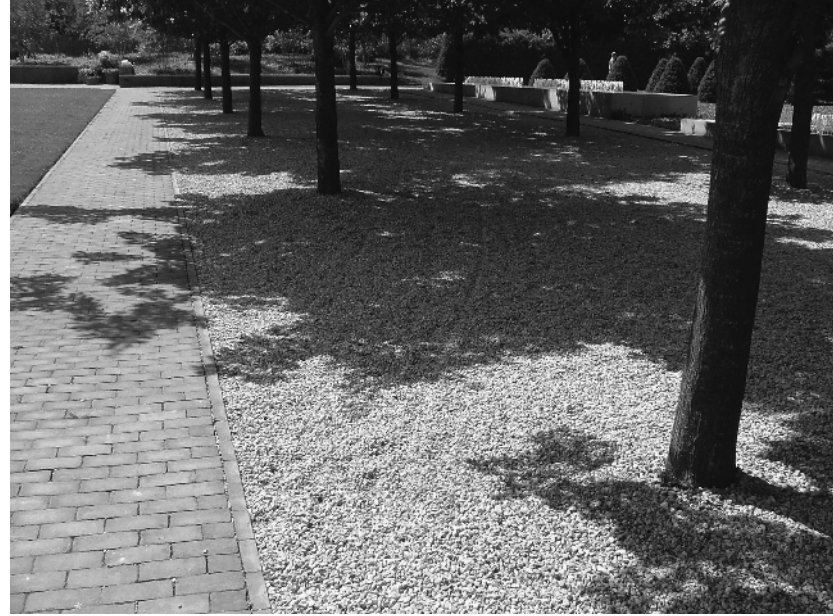
Figure 1-3 Serving as a mulch, this well-graded aggregate bed yields effective weed and moisture control.
