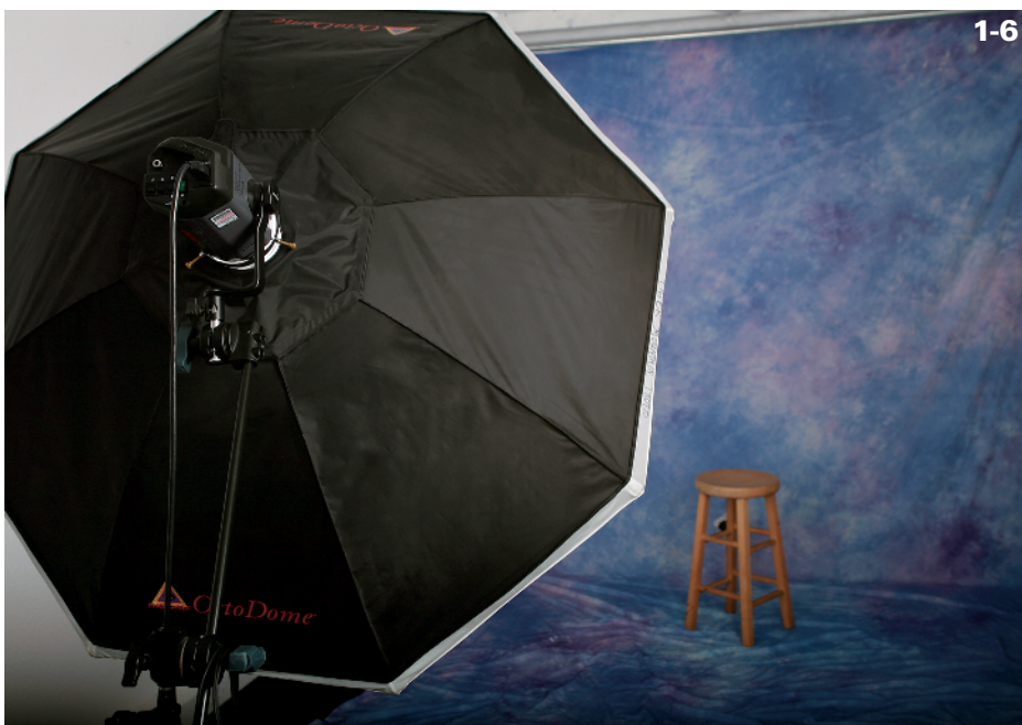
ABOUT THIS PHOTO A Photoflex Octodome softbox mounted on a Manfrotto tripod and boom, with a Bowens studio light, provides an adjustable modeling light and powerful flash that is triggered wirelessly from the camera. The back of the softbox (seen here) is black; the front of it is a white translucent material. ©Serge Timacheff
