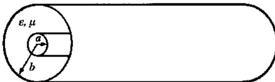
**FIGURE 1.16** The coaxial cable for illustrating the dependence of higher order modes on cross-sectional electrical dimensions.
