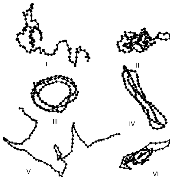
FIGURE 1.22 Typical conformations (I, random coil; II, molten globule; III, toroid; IV, rod; V, defect coil; VI, defect cylinder) of a 100-segment homopolymer generated by Monte Carlo simulations. (Source: Ref. [32].)
