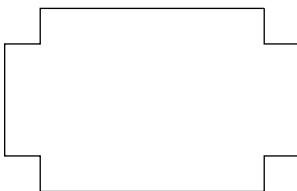
Figure 1-6: Cut squares from the corners.
