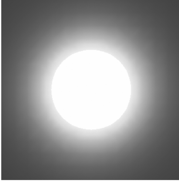
FIGURE 1.14 Density plots of coions (cations) around a positively charged spherical particle with y_0 = 2 at \kappa a = 1 . Calculated from n_+(r) = n \exp(-y(r)) with the help of Eq. (1.121). The darker region indicates the higher density and n_+(r) tends to its bulk value n far from the particle.
