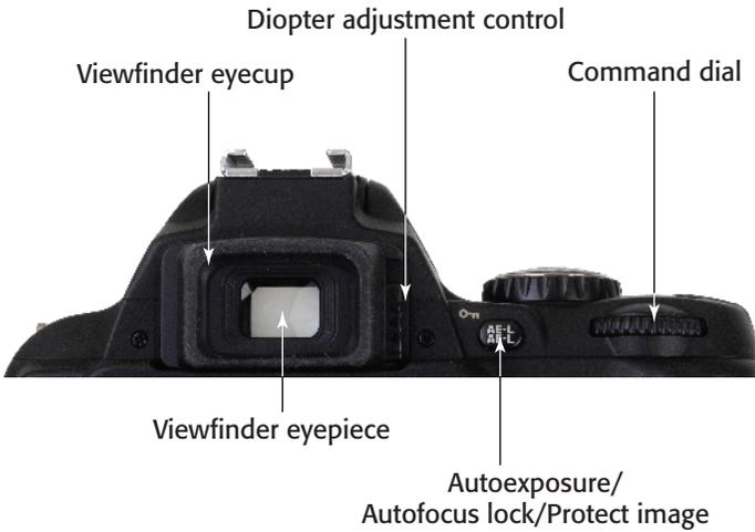
**1.13** Key components on the upper half of the back panel of the D40/D40x
