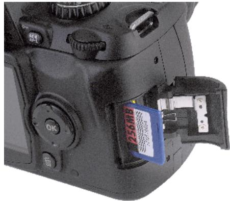
**1.7** A memory card fits into the slot on the side of the camera.
