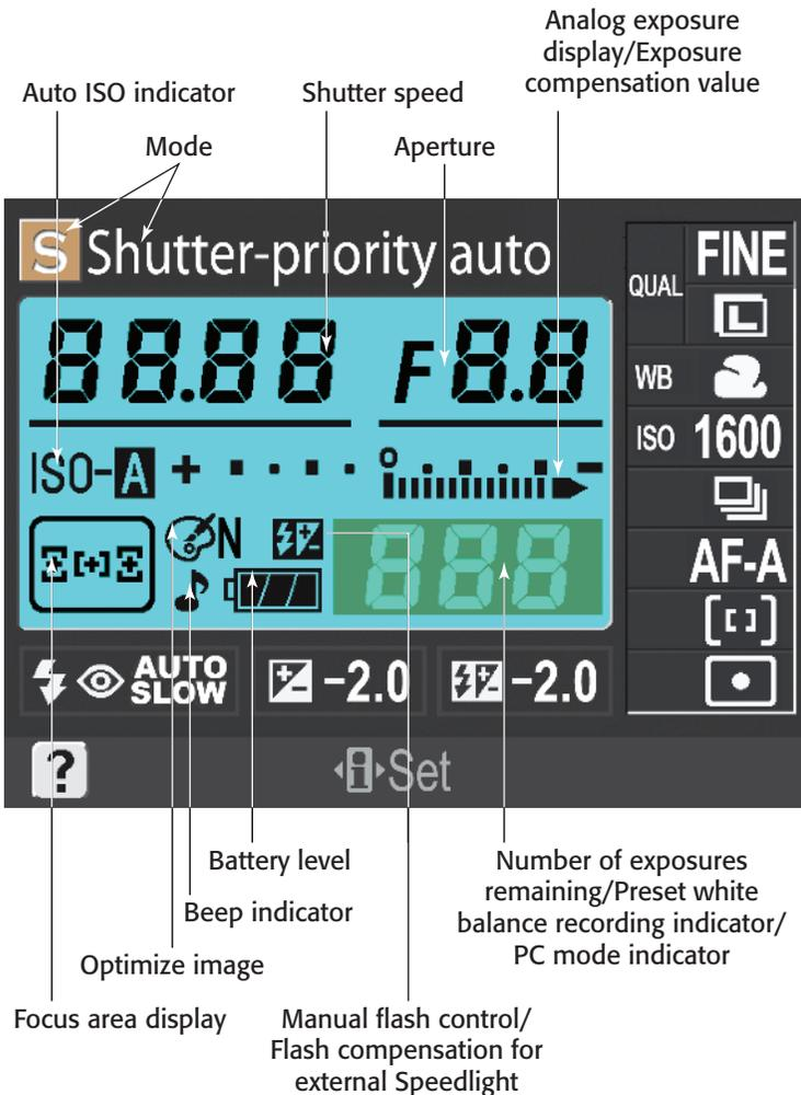
1.16 LCD readouts and indicators, part one
