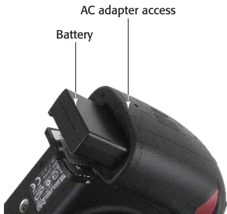
**1.8** A compartment in the bottom of the D40/D40x accepts a rechargeable battery and an optional AC adapter.
