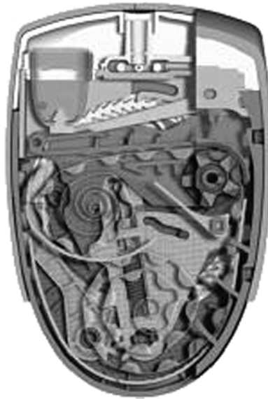
Figure 1.5 Cutaway diagram of a dry powder inhaler (DPI) showing the internal complexity of the device/container closure system and its many components. Many DPI components are plastic or elastomeric and therefore potentially capable of leaching. (Images provided by Valois Pharma.)
