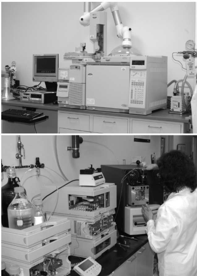
Figure 1.7 Typical GC/MS (top) and LC/MS (bottom) systems in common use in pharmaceutical development laboratories. Such systems are used to identify and quantify drug- and excipient-related impurities and metabolites, as well as extractables and leachables.
