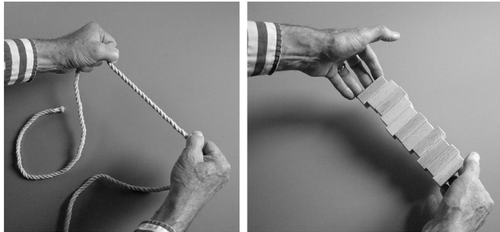
**Figure 1.10** Tension is pulling; compression is pushing. The rope at the left can resist only tension. The stack of small wooden blocks to the right cannot resist tension but can resist compression, even though the blocks are not connected to one another except by friction.
