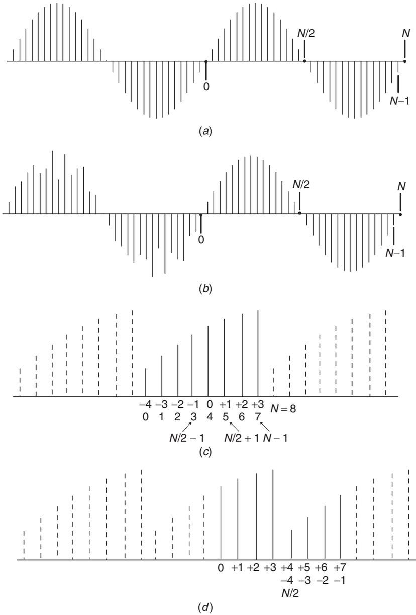
**Figure 1-1** Infinite sequence operations for wave analysis. (a) The segment of infinite periodic sequence from 0 to  $N - 1$ . The next sequence starts at  $N$ . (b) The Segment of infinite sequence from 0 to  $N - 1$  is not periodic with respect to the rest of the infinite sequence. (c) The two-sided sequence starts at  $-4$  or 0. (d) The sequence starts at 0.
