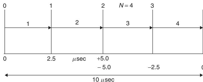
**Figure 1-4** A 10- $\mu\text{sec}$  time sequence with positive and negative time values.
