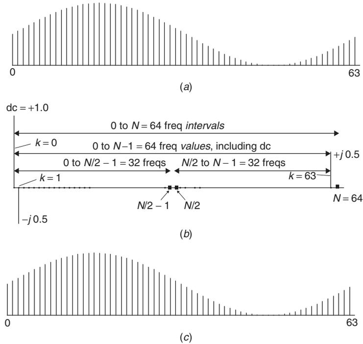
**Figure 1-2** Sequence (a) is converted to a spectrum (b) and recon-
