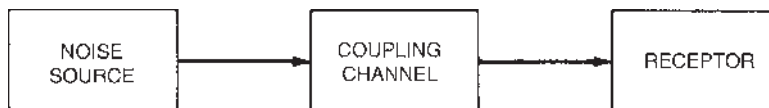
FIGURE 1-7. Before noise can be a problem, there must be a noise source, a receptor, and a coupling channel.
