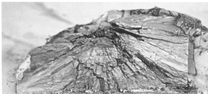
FIGURE 1. Post mortem examination of the titanium diboride "dwell target". The impact direction is from the top.
