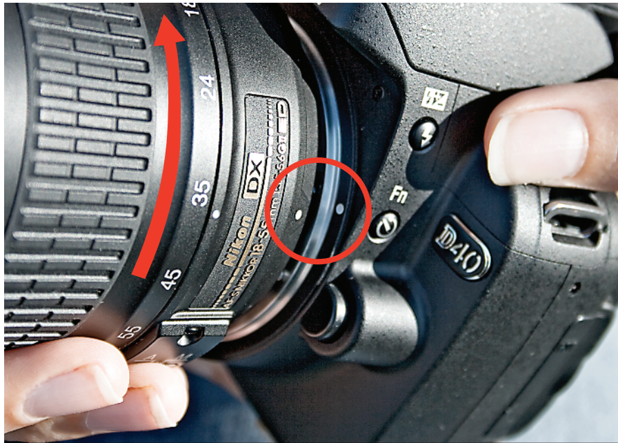
Figure 1-1: When attaching the lens, align the index markers as shown here.
