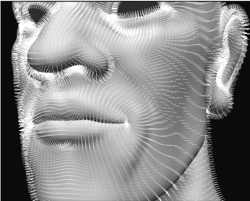
Figure 1.13 An image of a model in ZBrush with its normals visible. The normal is displayed as a line that shows which side of the polygon is pointing “out.”
