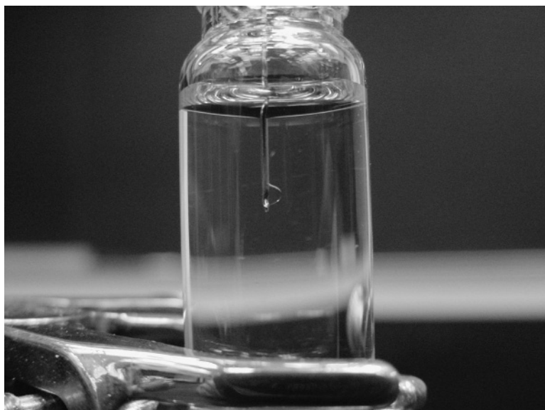
FIGURE 1.2. A 1- \mu\text{L} drop of octane suspended in aqueous solution on the tip of a Hamilton 701 GC syringe needle.
