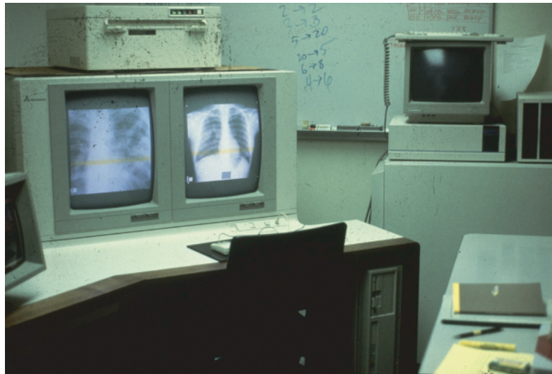
Figure 1.1v Early display system with two Megascan 2K monitors at UCLA.
