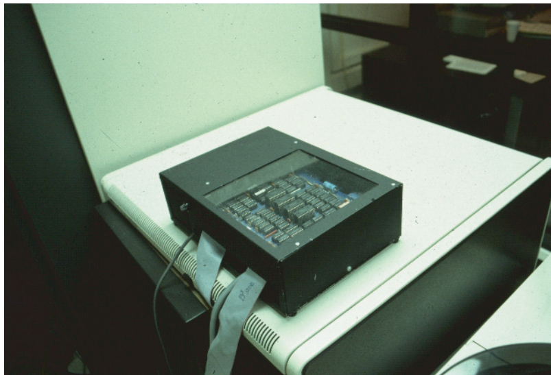
Figure 1.1p First interface box using the DR-11 W technology transmitting digital CR images out of the PCR-901 and PCR-7000 systems (Philips Medical Systems) to a PACS acquisition computer at UCLA. The concept allowing direct transmission of a full CR image to the outside world as input to PACS was the cornerstone of viewing direct digital projection image on a display monitor.
