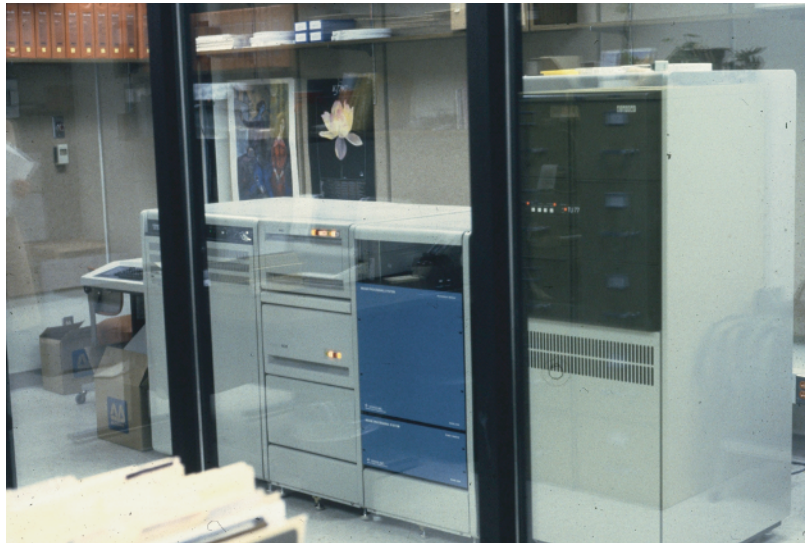
Figure 1.1t Gould DeAnza display controller (middle, blue) for a 1024-line 3-color display system (24 bits/pixel) with the VAX 750 (left) as the control computer.
