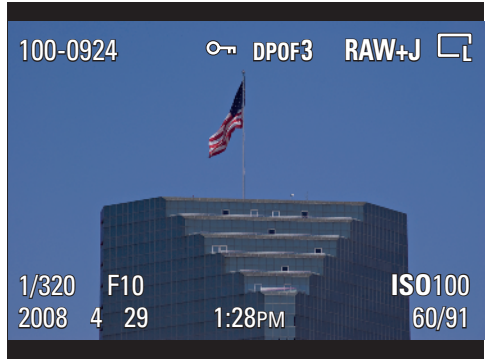
1.11 The screen in the Playback mode showing an image with the shooting data
