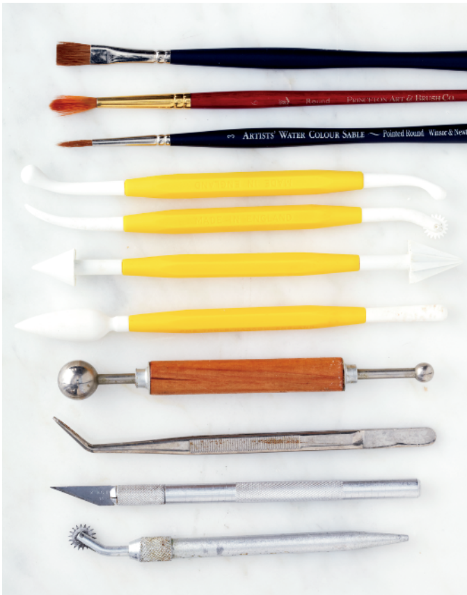
Brushes and modeling tools, from top to bottom: 1/4-in (6 mm) flat paint brush, #5 round brush, #1 paint brush, dogbone tool, quilting wheel/veiner tool, cone and serrated tool, trumpet tool, large and small ball tool, angular tweezer, X-acto knife, metal quilting wheel.
